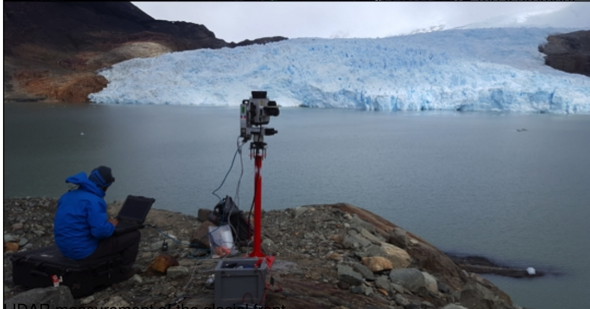
LIDAR measurement of the glacial front
